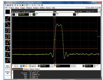
Figure 5. 100 ps pulse with 17 ps risetime.
