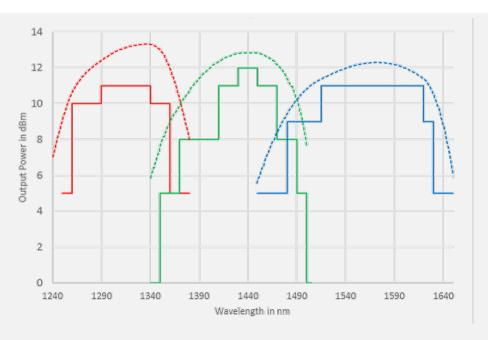
Figure 5. Wavelength coverage of options 113 (red), 114 (green) and 216 (blue). Typical maximum output power (dotted line) vs. specified output power (solid lines)
