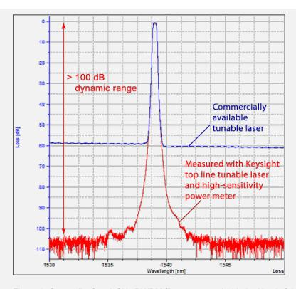
Figure 3. Crosstalk of a 50 GHz DWDM filter, measured with the N7747C high-sensitivity power meter
