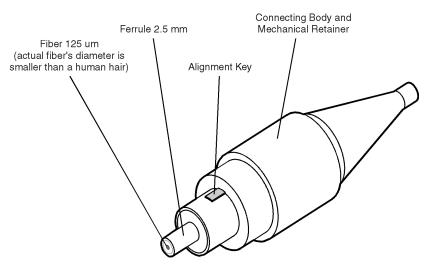
Figure 5-1. Basic components of a connector.
