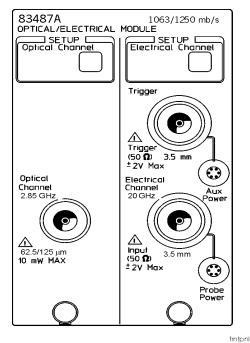
Front panel of the plug-in module.
