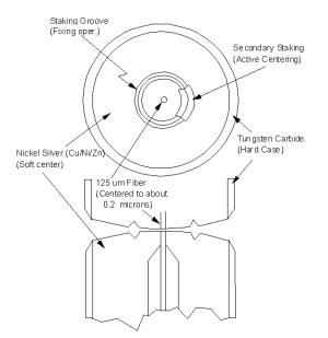
Figure 5-3. Cross-section of the Diamond HMS-10 connector.
