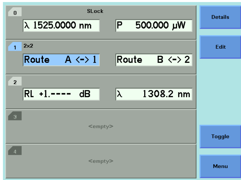
Figure 144 Optical Switch module, User Interface Overview display
