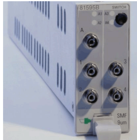
Figure 143 Keysight 81595B Optical Switch module ( 1x4, angled contact connectors)
