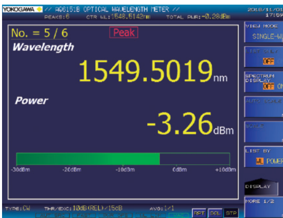
The horizontal bar graph easily identifies the optical power variation and flatness of the signal.
