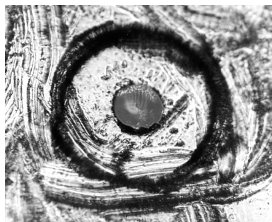
Figure 6 Damage from improper cleaning.
